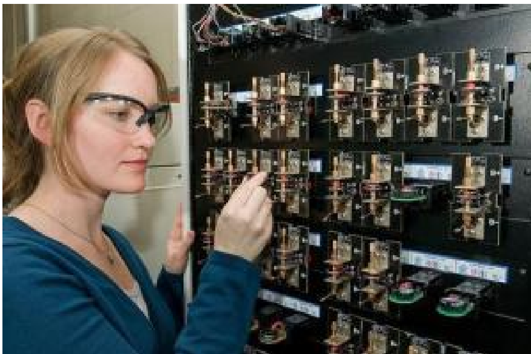
Argonne researcher Lynn Trahey loads a coin-sized cell on a testing unit used to evaluate electrochemical cycling performance in batteries. (Credit: Photo by Wes Agresta / Courtesy of Argonne National Laboratory)
